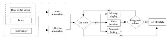
Figure 2. Structure of the car door collision avoidance system
