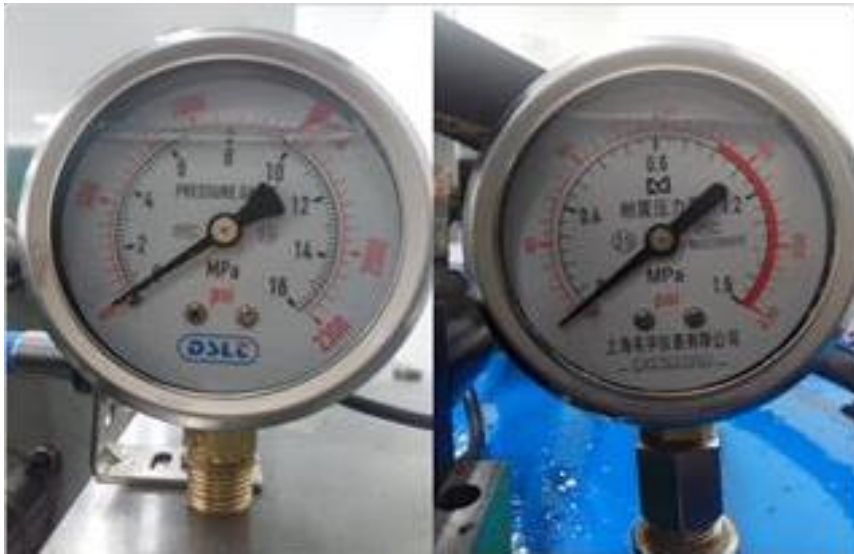
Fig 6. Comparison diagram of pressure gauge before and after commissioning
